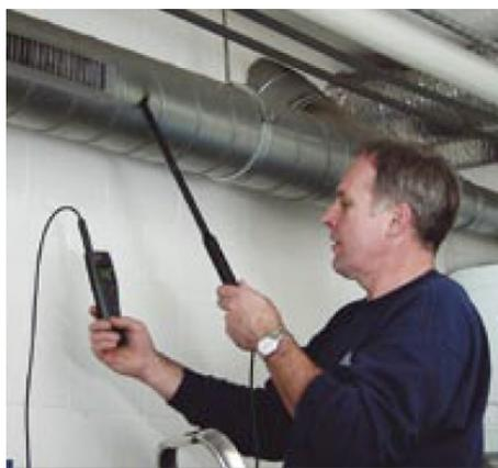
*A check can help in assessing whether a hygrometer is functioning as expected, and whether repair or recalibration is needed.*
